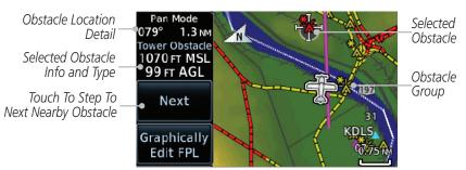
Figure 8-23 Point Obstacle Detail
