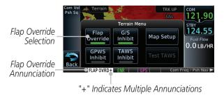
Figure 10-40 TAWS-A Page Menu and FIT Flap Override Annunciation
