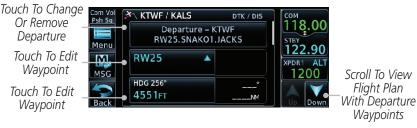
Figure 6-7 Flight Plan View of the Selected Departure
