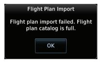
Figure 4-77 Flight Plan Import Fault - Catalog Full
