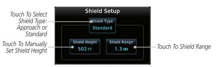
Figure 9-29 TCAD 9900B Shield Setup for En Route, Standard, and Terminal
