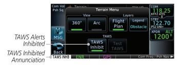
Figure 10-14 TAWS-B Alerting Disabled (TAWS Inhibited) Annunciation
