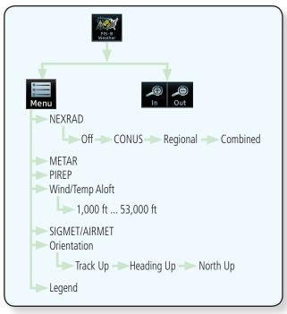
Figure 11-71 FIS-B Weather Functional Diagram
