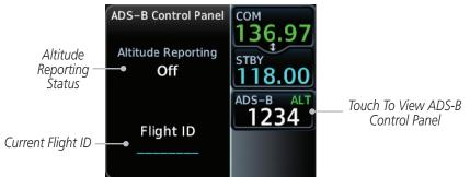
Figure 2-13 ADS-B Control Panel
