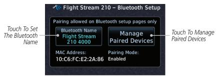
Figure 15-51 Bluetooth Setup for Flight Stream
