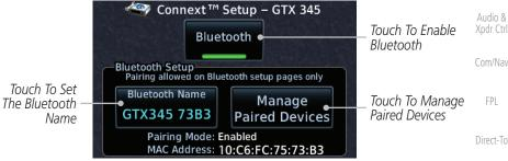
Figure 15-56 Connext Setup for GTX 345
