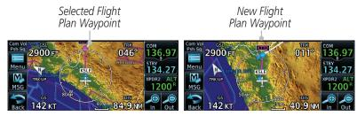
Figure 4-14 Flight Plan Before and After New Waypoint Inserted
