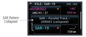
Figure 4-31 SAR Pattern Collapsed in Flight Plan
