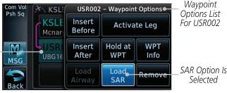
Figure 4-28 Active Flight Plan with Load SAR Option
