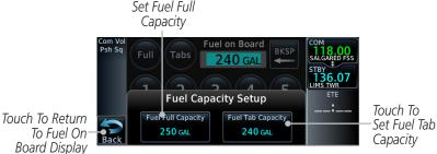
Figure 1-14 Fuel Capacity Setup Page
