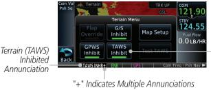
Figure 10-36 TAWS-A Alerting Disabled (TAWS Inhibited) Annunciation
