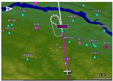
Figure 8-57 Active Flight Plan Leg Prior to Holding Pattern
