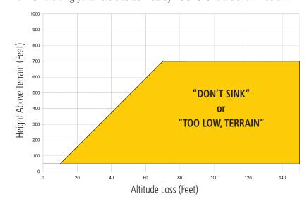
Figure 10-42 Negative Climb Rate (NCR) Altitude Loss
