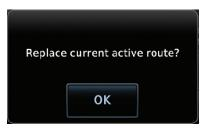
Figure 4-52 Touch OK to Invert and Activate the Selected Flight Plan
