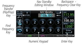
Figure 3-6 Nav Standby Frequency Numeric Keypad
