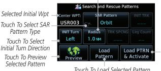
Touch To Load Selected Pattern To The Active Flight Plan
