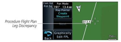
Figure 4-16 Procedure Flight Plan Leg Position Difference
