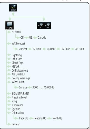
Figure 11-3 SiriusXM Weather Page Functional Diagram
