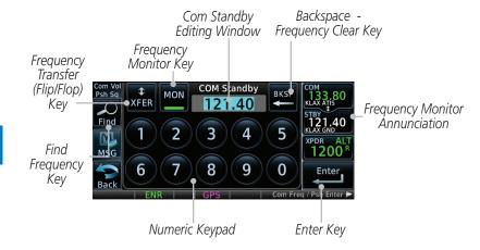
Figure 3-5 Com Standby Frequency Numeric Keypad
