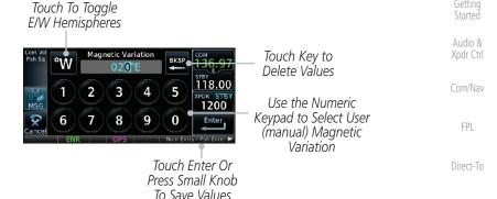
Figure 15-42 Numeric Keypad for Setting Manual Magnetic Variation
