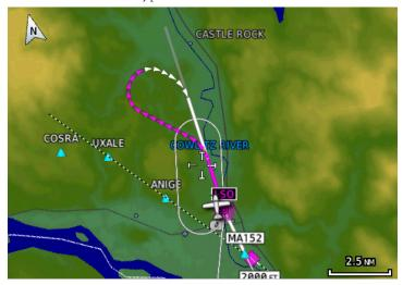
Figure 8-53 Active Procedure Turn
