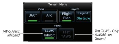
Figure 10-9 TAWS-B Alerts Inhibited Selected
