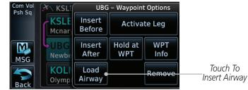
Figure 4-19 Select Load Airway from the Waypoint Options
