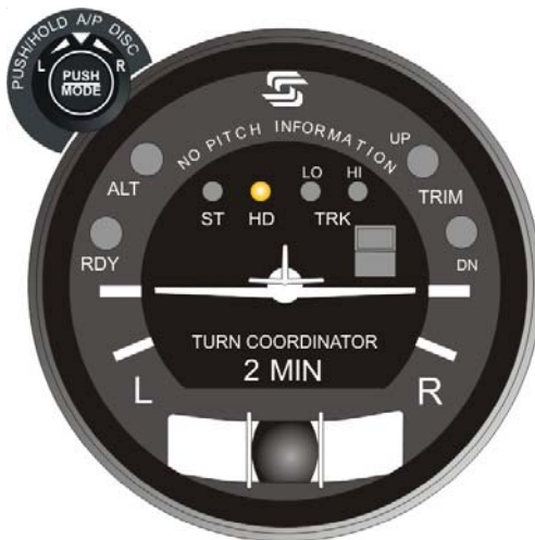
Fig. 2-18. AP Display, HD Mode Engaged (System Twenty)
