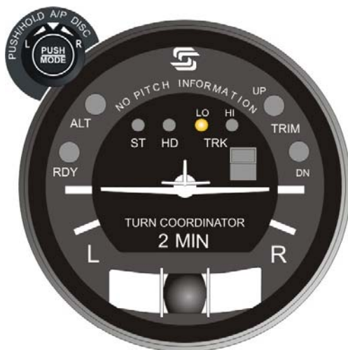
Fig. 3-3. AP Display, LO TRK Mode Engaged
