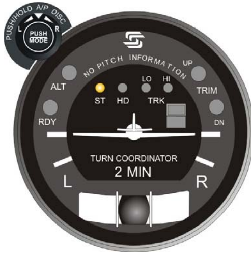
Fig. 2-21. AP Display, ST Mode Engaged (System Thirty)
