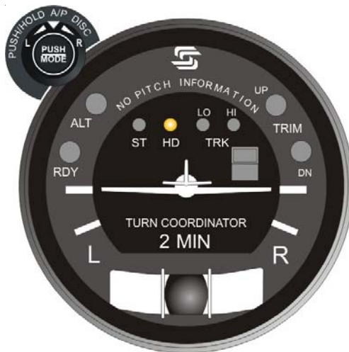
Fig. 2-22. AP Display, HD Mode Engaged (System Thirty)
