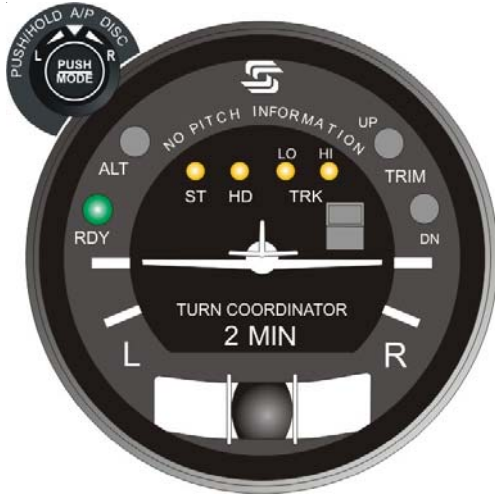
Fig. 2-1. AP Display, RDY, ST, HD, LO TRK, HI TRK Lamps Illuminated at Power-Up (System Twenty)
