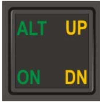
Fig. 2-13. ALT HOLD ON/OFF Switch Display, ALT ON, UP, and DN Lamps Illuminated at Power-Up (System Thirty ALT)
