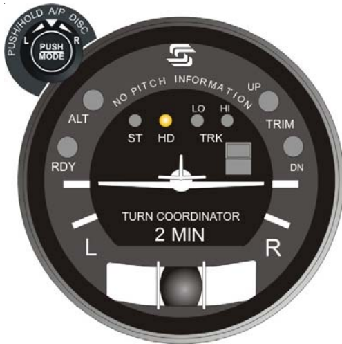
Fig. 3-2. AP Display, HD Mode Engaged
