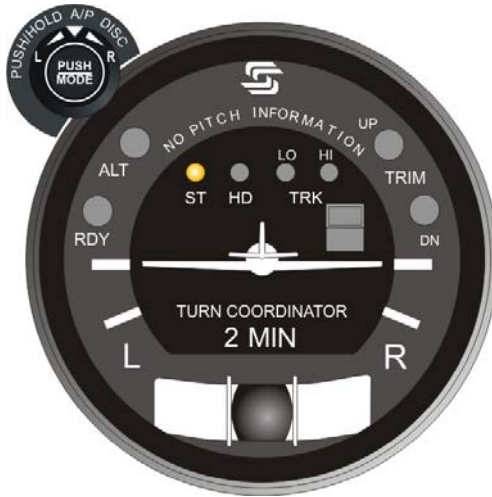
Fig. 2-17. AP Display, ST Mode Engaged (System Twenty)
