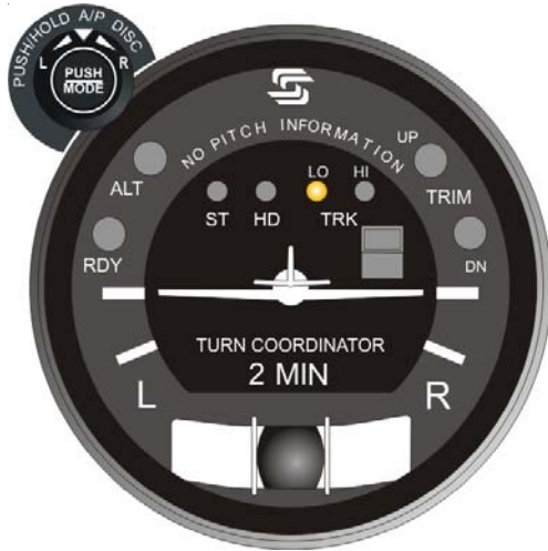
Fig. 2-19. AP Display, LO TRK Mode Engaged (System Twenty)
