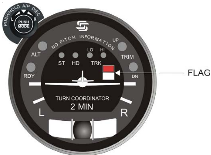
Fig. 2-12. AP Display, Low Voltage Flag (System Thirty)
