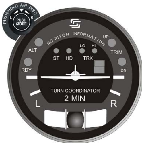
Fig. 2-11. AP Display, Turn Coordinator Failure (System Thirty)
